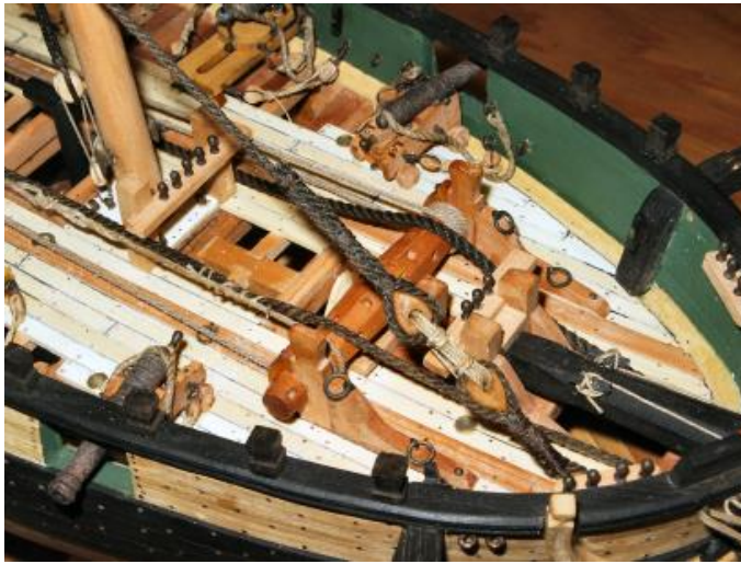
Model of the Oneida as armed in 1813, without the pivot gun or platform and showing the two foremost gun ports, originally occupied by 24-pound carronades, now with 6-pound cannon. The location of the windlass is probable but not confirmed. Model by Clayton Nans; photograph by the author.
