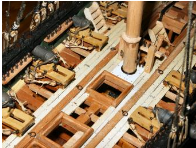
Model of the Oneida showing four of her starboard 24-pound carronades as well as two carronades on the port side. Model by Clayton Nans. Photograph by the author.
