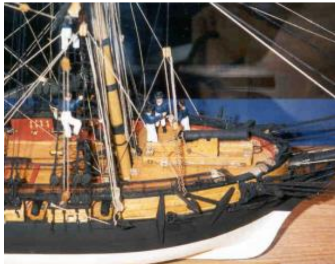
Another model of the Oneida showing the as-designed 32-pound pivot gun on the forecastle platform. Model by Patrick Wilder; photograph by the author.
