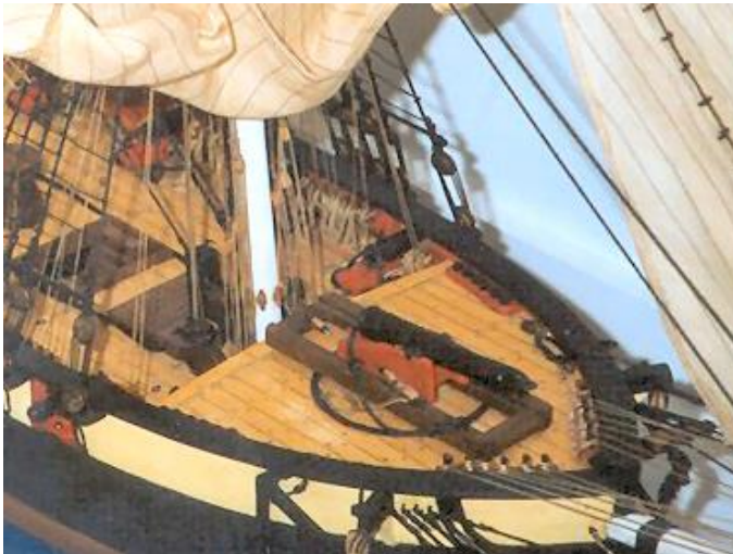
Model of the Oneida showing the as-designed 32-pound pivot gun on the forecastle platform. The carronades are incorrectly mounted on truck (wheeled) carriages instead of slides. Model at the Sackets Harbor Battlefield State Historic Site, Sackets Harbor, NY; photograph by the author.
