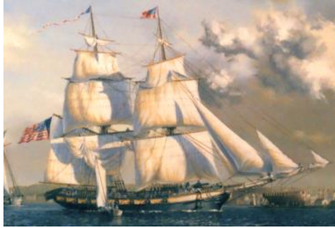
The Oneida as designed, with 16, 24-pound carronades and a 32-pound pivot gun forward, as it would have appeared sailing off Sackets Harbor. Painting by Peter Rindlisbacher.
